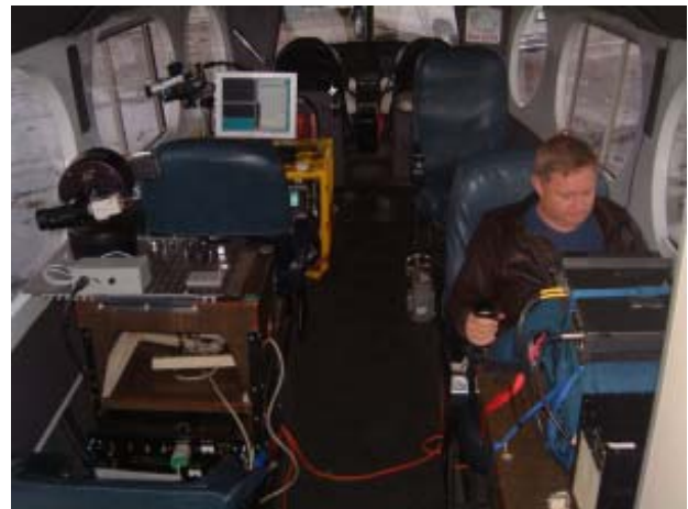
Figure 5 - IR detection suite on left, consisting of visible camera on gimbal, operator station, detection camera. WesCam operator station on right.
