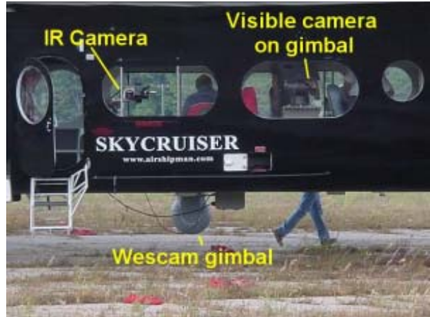
Figure 4 - Installation in airship.
