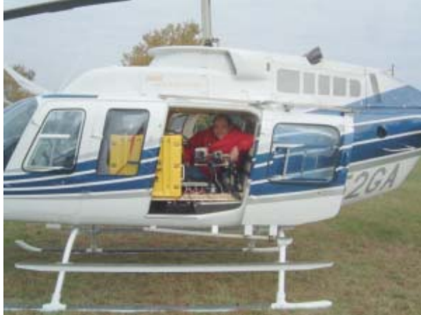
Figure 1 - First flight. Processor is strapped down in yellow rack, IR and visible cameras are on stand, and batteries are on floor under plywood frame.
