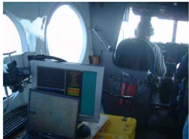
Figure 6 - Test flight with IR detection suite, moving map geolocation on laptop.
