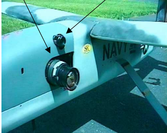
Figure 2. Integration of Viper Sensors with NRL Sparrow UAV
